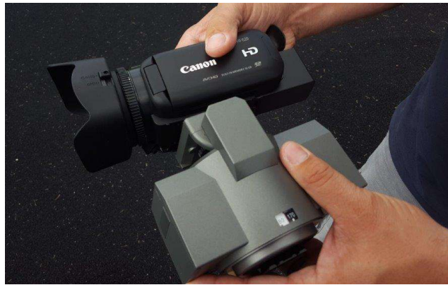
10. Attach camcorder to pan tilt unit.
