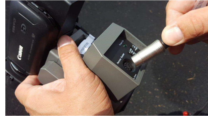
12. Plug in pan tilt cord to back of unit.
