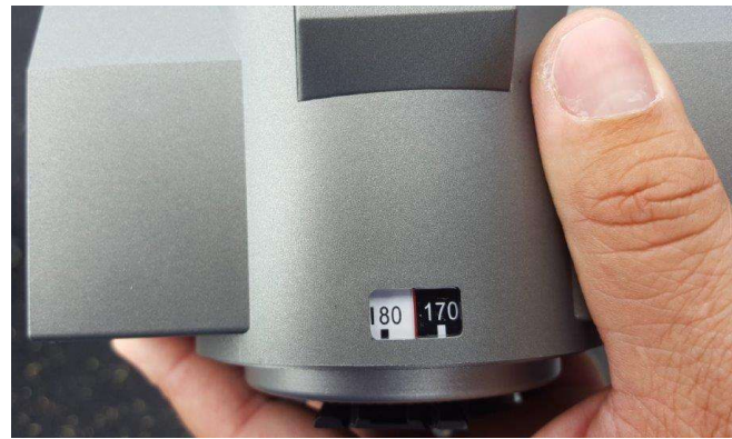
11. Turn unit to "340" and "A" to center unit at 170. Once centered, move switch back to "M". Make this a habit before every use. Also ensure mount plate underneath is tight before use.
