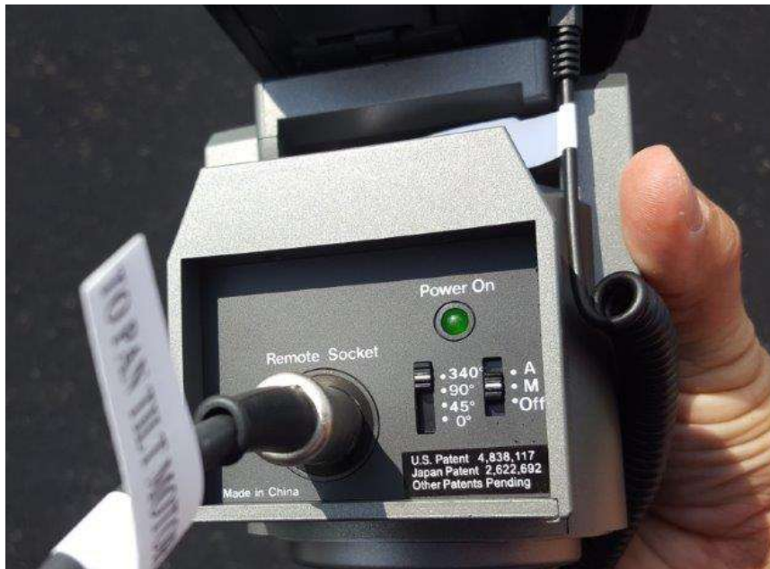
13. Your unit should look like this with the two selector switches on "340" and "M". The "Power On" light should also be illuminated. Unit runs on 4 AA batteries that should be replaced every 2 or 3 games.
