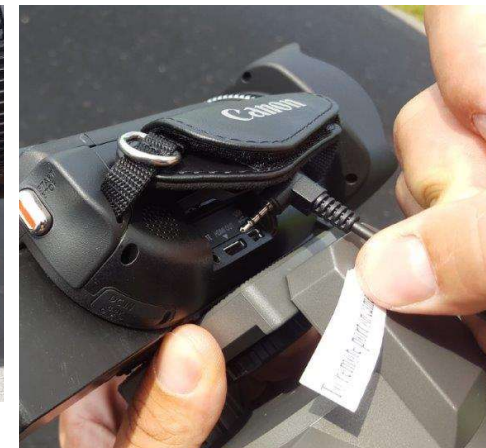
15. Gently plug small 2.5mm cable into remote port on camera.
