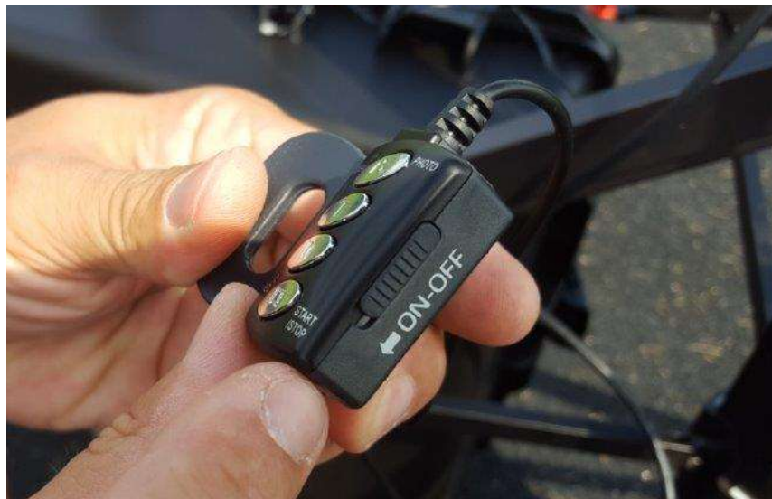
27. Slide power switch on side of LANC remote down to power on camcorder. The power light will illuminate on remote.
